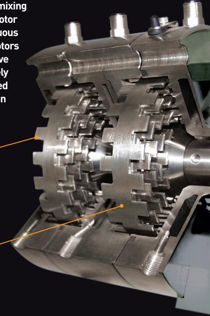
For food manufacturing applications, the entire machine is made from high-grade 316 stainless steel – including the mixer, the pump and all the pipework and fittings. The electric motors that drive the pump and rotors are fitted with variable output gears and inverter controls.
