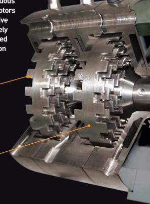
For food manufacturing applications, the entire machine is made from high-grade 316 stainless steel – including the mixer, the pump and all the pipework and fittings. The electric motors that drive the pump and rotors are fitted with variable output gears and inverter controls.
