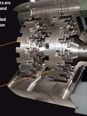
CR mixers can be used for the homogenous mixing of liquid products, or the production of foam by aeration of a liquid product, with the further capability of also injecting up to 4 additives into the mixer during processing, 2 at the beginning of the mix, and 2 before the end, with the further option of post-blending of products into the product mix or foam.
